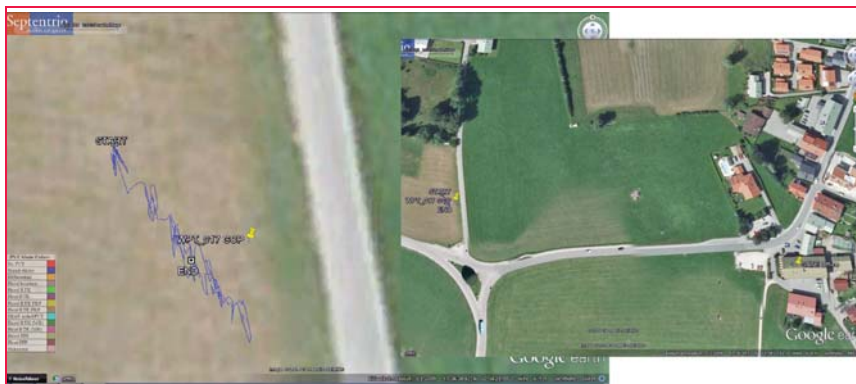
Figure 11: Position fixed at GATE Central Point and results exported to Google Earth: The yellow pins marks the reference position on WPT_017 GATE Central Point; the blue trace shows all positions measured between START and END of a 3 minutes measurement; deviations were observed to lie within a 5m radius
